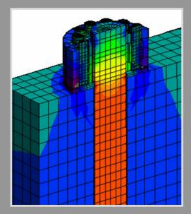
With **StretchHold** the whole applied preload is used for elongating the bolt, friction loss does not exist, therefore a higher precision is obtained; higher preloads per bolt. Due to this fact, with **StretchHold** the number of bolts in a joint union can diminish, saving material and eliminating machining.
